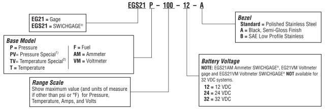
NOTE: The EG21PV-80-12, 24 or 32-A is designed to read senders with a resistance curve of 9.5 to 182 $\Omega$ , which are commonly supplied as standard senders on Deutz and VW Engines.
