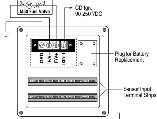
Terminal 1-15 Class "B" Sensors-Lockout.
