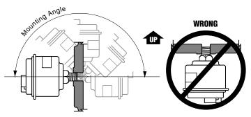
**3.** Locate the unit in place and secure it by tightening the 1/8-27 NPT fitting into the desired location (do not overtighten). **DO NOT TWIST CASE.**
