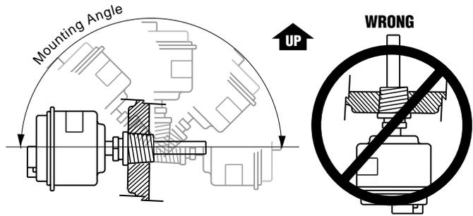
2. Install the TSB switch in the engine water jacket location recommended by the engine manufacturer.
