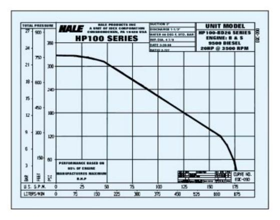
Impeller Diameter: 4-7/8 inches. Suction: 2 inch FNPT Discharge: 1-1/2 inch FNPT Length: 32.3 inches (859 mm) Width: 16.5 inches (419 mm) Height: 29.55 inches (751 mm) Weight: 315 lbs (143 kg)
