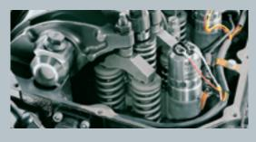
Thanks to the *injection pressures of up to 1600 bar* of Common Rail and EUI systems and to the flexibility of electronic control over all air and fuel parameters, the combustion process is optimized and *gas and acoustic emissions are contained* below the limits prescribed by current and future *EPA*, *EURO and CE standards*, which for NEF engines are also assured by the option of equipping them with *traditional injection pumps*.
